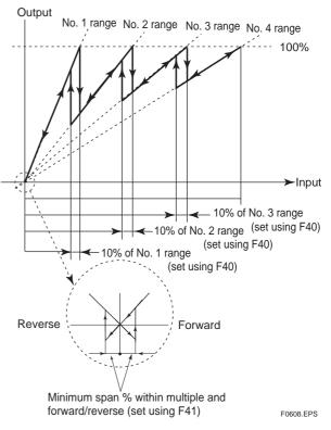
Figure 6.4.1 Multiple Ranges and Hysteresis Widths
